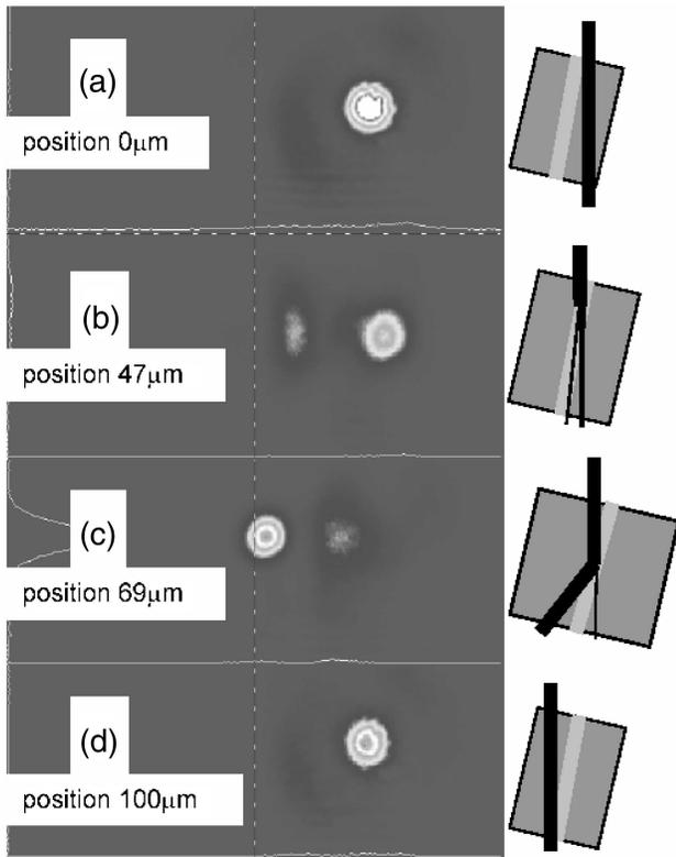
Fig. 3. Collage of beam geometries (right-hand side) and output beam distributions for several relative sample input beam positions. (Second-harmonic generation output spatial distribution is shown.) Input intensity,  $6 \text{ GW/cm}^2$ ; incidence angle, approximately  $0.5^\circ$ . The transverse beam positions given are relative to (a) (at  $0 \mu\text{m}$ ).
