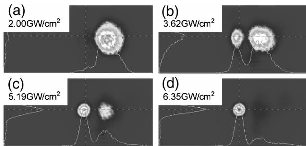
Fig. 4. Output beam distributions for beam incidence on the boundary in the middle of the sample for increasing input intensities. (Second-harmonic generation distribution at the end of the sample is shown.)
