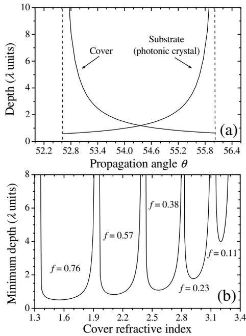
FIG. 5. (a) Evanescent wave penetration depth,  $\Gamma_{es}$ ,  $\Gamma_c$  into a photonic crystal substrate and cover for a structure with filling factor  $f = 0.74$  and a cover  $n_c = 1.55$ . (b) Minimum depth  $\Gamma_{es,min}$  of the evanescent wave inside the photonic crystals as a function of the cover refractive index, for the different filling factors considered in Fig. 4.
