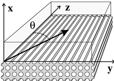
FIG. 1. Sketch of the particular structure analyzed here, consisting of a cover made of an isotropic material and a substrate photonic crystal. The lattice constant  $a$  of the 2D photonic crystal is much smaller than the excitation wavelength. The concept holds for different cell shapes and for general anisotropies.
