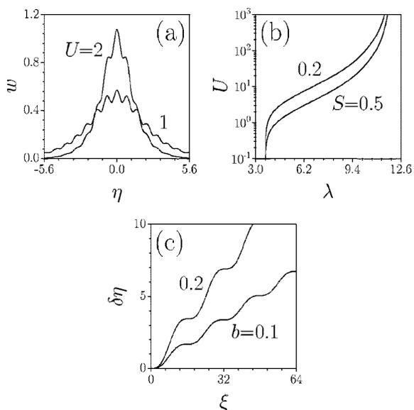
Fig. 2. (a) Soliton profiles supported by an undistorted lattice at  $E=12$ ,  $S=0.2$ . (b) Soliton energy flow versus propagation constant at  $E=12$ . (c) Trajectory of the integral center of a soliton with  $U=1$  in a distorted lattice at  $\beta=4.1$ ,  $E=12$ ,  $S=0.2$ .
