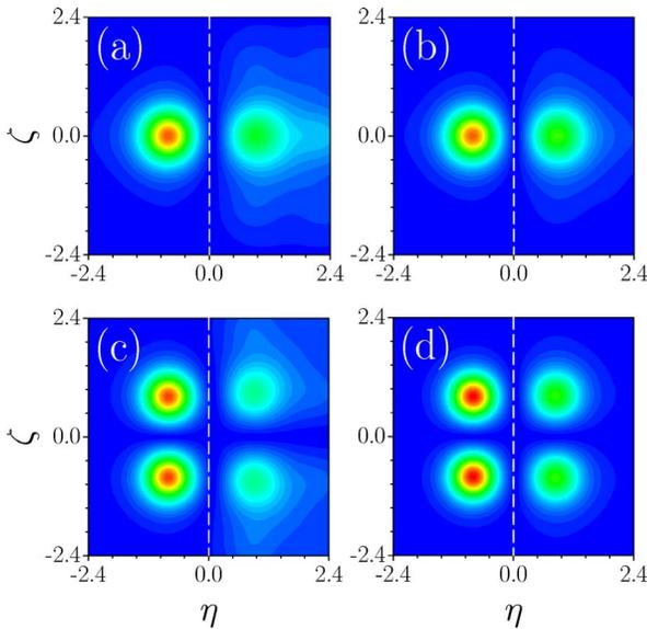
Fig. 1. (Color online) Field modulus distributions of dipole-mode surface solitons corresponding to (a)  $b=3.45$  and (b)  $b=4.05$  at  $p=4$ ,  $\delta p=2$  and quadrupole-mode solitons corresponding to (c)  $b=5.33$  and (d)  $b=7.5$  at  $p=4$ ,  $\delta p=4$ . Vertical dashed lines indicate the interface position.
