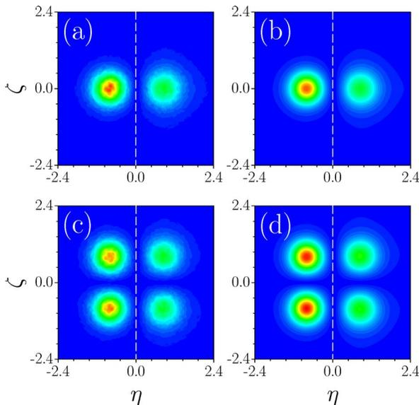
Fig. 3. (Color online) Stable propagation of a dipole-mode soliton with  $b=7$  and a quadrupole-mode soliton with  $b=7.5$  in the presence of white input noise with variance  $\sigma_{\text{noise}}^2=0.01$ . Field modulus distributions are shown at (a), (c)  $\xi=0$  and (b), (d)  $\xi=256$ . In all cases  $p=4$ ,  $\delta p=4$ .
