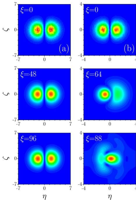
Fig. 2. (Color online) Propagation dynamics of slightly perturbed dipole-mode solitons with (a)  $b=3$  and (b)  $b=12$ .
