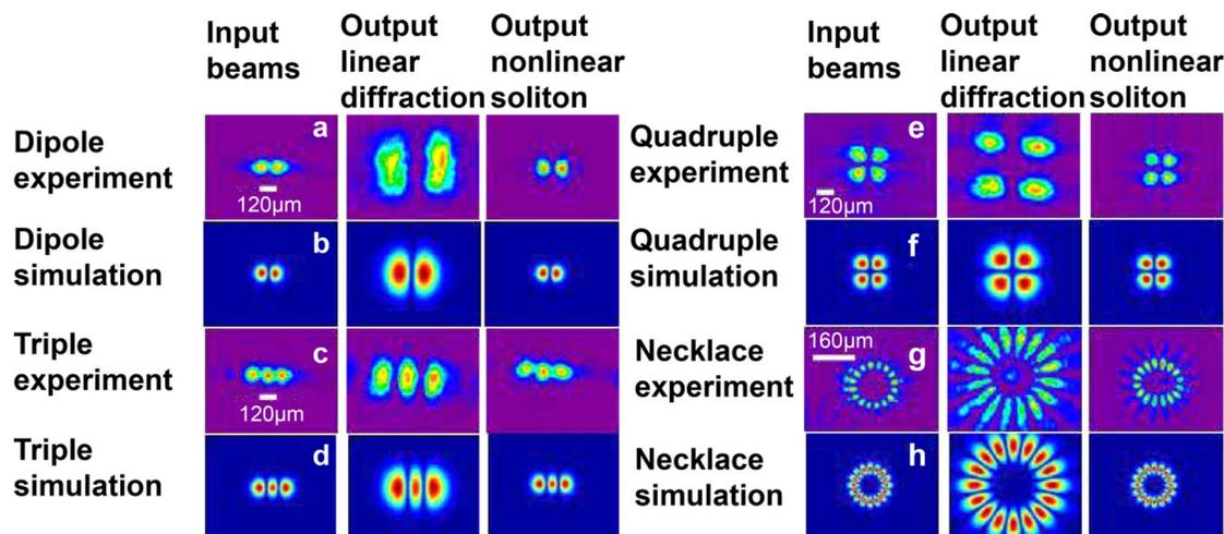
Fig. 1. (Color online) Experimental and theoretical observations of complex scalar solitons in the form of, a, b, dipole solitons; c, d, tri-pole solitons; e, f, quadrupole solitons; g, h, necklace solitons. Left-hand columns, input beams; central columns, output beams after linear diffraction broadening for 84 mm of propagation; right-hand columns, high-power self-trapped output beams after the same distance.
