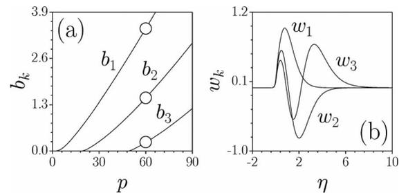
Fig. 2. Linear surface modes supported by the refractive index profile induced by thermal wave at  $t=\tau/8$  for  $\tau=16$ . (a) Propagation constants versus modulation depth  $p$ . (b) Profiles of the first three linear modes at  $p=60$  corresponding to points marked by circles in (a).
