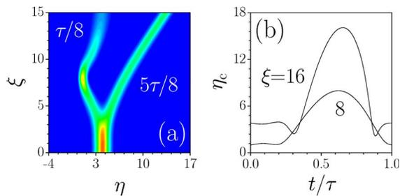
Fig. 3. (Color online) Steering of near-surface soliton  $q(\eta, 0) = \text{sech}(\eta - \eta_0)$  by thermal wave at  $\eta_0 = 4$ ,  $\tau = 64$ , and  $p = 5.5$ . (a) Superimposed field modulus distributions for solitons in the time moments  $t_1 = \tau/8$  and  $t_2 = 5\tau/8$ . (b) Soliton center displacements versus time at different propagation distances.
