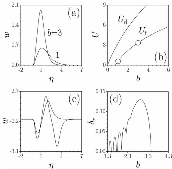
Fig. 4. Nonlinear surface modes supported by thermally induced refractive index profiles at  $t = \tau/8$  for  $\tau = 16$ . (a) Profiles of fundamental modes with different  $b$  at  $p = 20$ . (b) Energy flow versus  $b$  for fundamental and dipole modes at  $p = 20$ . Points marked by circles correspond to profiles shown in (a). (c) Profiles of dipole and triple-mode solutions at  $b = 4$ ,  $p = 60$ . (d) Real part of perturbation growth rate for triple-mode solution at  $p = 60$ .
