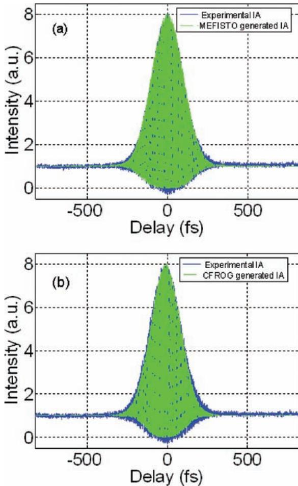
Fig. 4. Interferometric autocorrelations. (A) from MEFISTO and (B) from CFROG.
