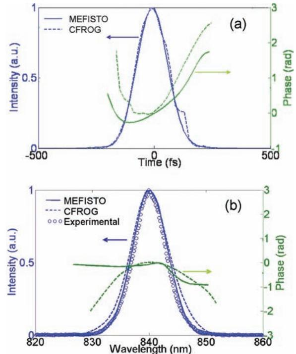
Fig. 5. Retrieved phase and intensity profiles of the pulse at the sample plane of the microscope obtained with MEFISTO (solid line) and standard CFROG procedure (dashed line): (A) temporal intensity and phase. The temporal width (FWHM) of the pulse at the sample plane is 163 fs. (B) The measured spectrum (circles) and the retrieved spectral intensity and phase profiles.
