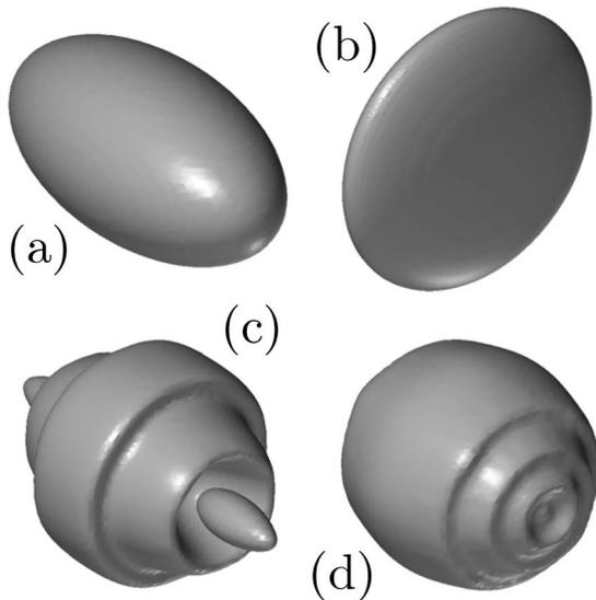
Fig. 1. Isosurface plots showing output patterns after propagation at  $\xi=2$  of input Gaussian signals in linear tandem structures with (a), (b)  $d=20$ ; (c)  $d=0.8$ ; and (d)  $d=0.4$ . In (a) the dispersion in the central domain is set to  $\beta=-2$ . In (b)–(d),  $\beta=-0.1$ .
