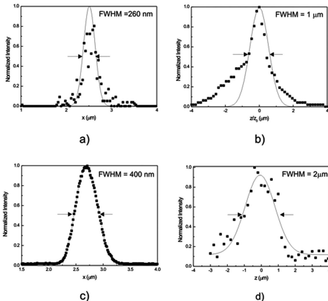
FIG. 3. Cross-sections of the measured PSFs (a) along the  $x$ - and  $z$ -axis (a and b, respectively) in the confocal mode and along the  $x$ - and  $z$ -axis in the TPF mode (c and d, respectively). The depicted curve is a Gaussian fitting to the obtained data. The diameters of the beads were 200 nm.
