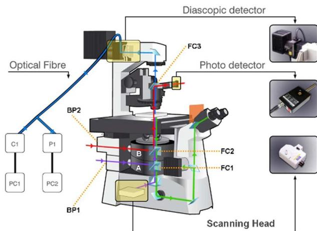
FIG. 2. (Color online) An artist's impression of the multimodal microscope system with its various light paths. Green light path-backward detected fluorescence, violet light path-epifluorescence and confocal excitation, blue light path-forward propagating SHG signal, red light path-NIR excitation, PC-computer, C1-confocal microscope control box, P1-PMT module 1, A-filter turret A, B-filter turret B, BP-back port, and FC-filter cube.
