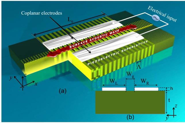
FIG. 1. (Color online) (a) Basic structure of ASL based-on ZX-cut PPLN with coplanar aluminum electrodes configuration. (b) Side view ( $yz$ -plane).
