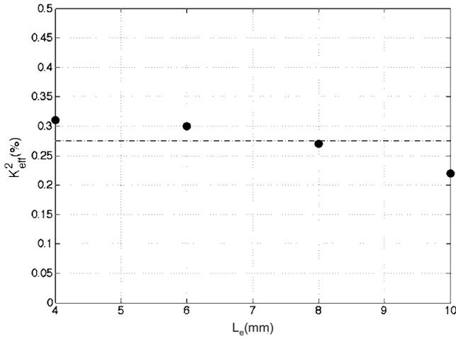
FIG. 4.  $K_{\text{eff}}^2$  as a function of the electrode length ( $L_e$ ), with dashed-line denoting the average  $K_{\text{eff}}^2$ .
