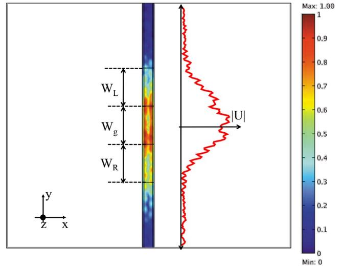
FIG. 5. (Color online) Top view of normalized magnitude of elastic displacements at a frequency of 252.97 MHz.
