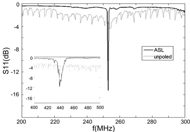
FIG. 2.  $S_{11}$  vs  $f$  for ASL with length  $L_e=10$  mm. Inset shows the corresponding longitudinal bulk wave response.
