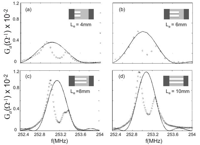
FIG. 3. Conductance ( $G_a$ ) (circles) of the ASL samples with different electrodes length. Solid lines denote the corresponding fitting curve.
