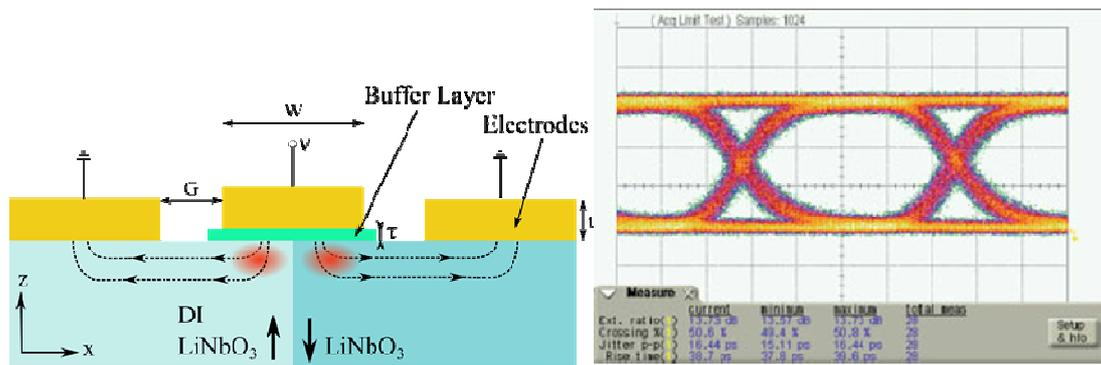
**Figure 2.** Cross section of an ultra-low voltage modulator (left) and typical eye diagram at 10 Gb/s (right)
