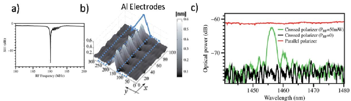
**Figure 1.** Typical response for an AO based superlattice SAW device based on DI with coplanar electrodes: a) RF S11 response, b) profile displacement of SAW measured by interferometric technique and c) low-power AO modulator performance.
